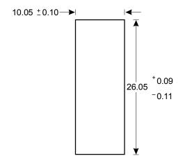
According to the dimensions and tolerances indicated in the diagram, which of the following actual dimensions is acceptable for this piece?
